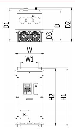
$\begin{array}{lll} D & = 246.6 \\ H1 & = 460 \\ W & = 222.8 \\ W1 & = 140 \\ Weight in (KG) = 12.68 \end{array}$
